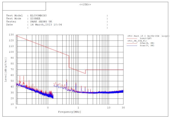
Result : The emissions 9 kHz to 30 MHz were 20 dB lower than the limit
