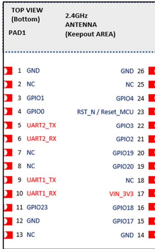
Figure 4-4 Interface UART Pin Assignments (Top View)
