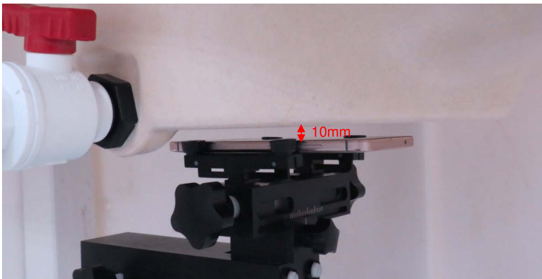
Picture 7: Front Side, the distance from handset to the bottom of the Phantom is 10mm
