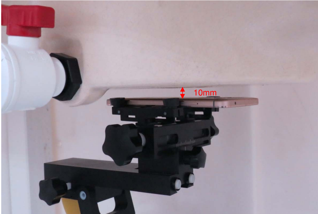
Picture 6: Back Side, the distance from handset to the bottom of the Phantom is 10mm
