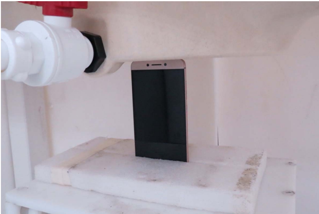
Picture 17: Top Side, the distance from handset to the bottom of the Phantom is 0mm
