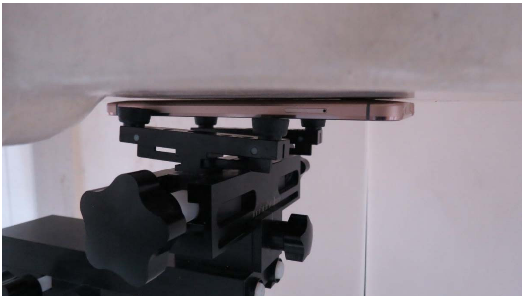
Picture 14: Back Side, the distance from handset to the bottom of the Phantom is 0mm
