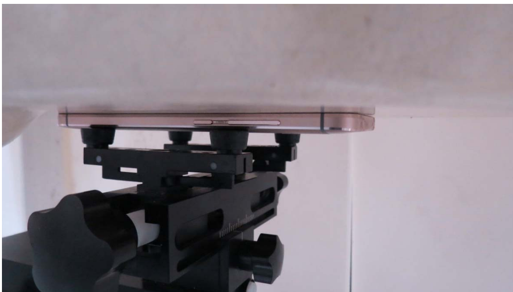
Picture 15: Front Side, the distance from handset to the bottom of the Phantom is 0mm
