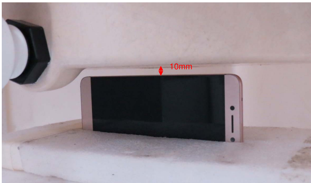
Picture 10: Left Side, the distance from handset to the bottom of the Phantom is 10mm
