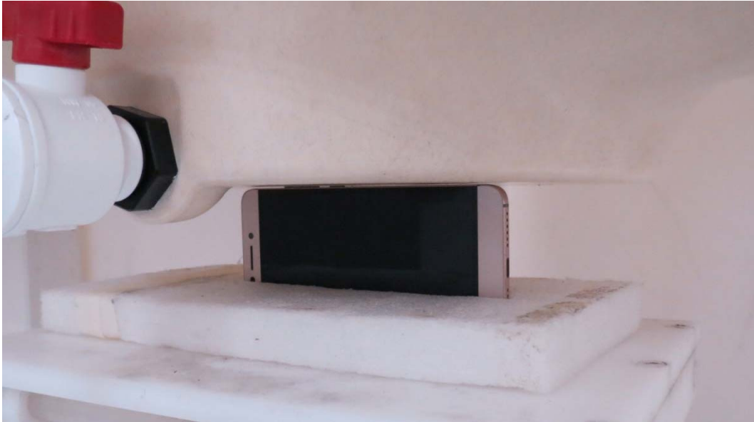
Picture 16: Right Side, the distance from handset to the bottom of the Phantom is 0mm
