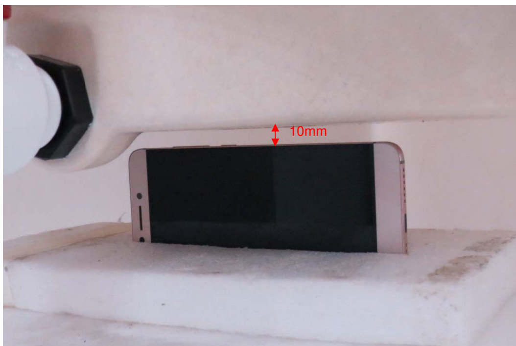
Picture 11: Right Side, the distance from handset to the bottom of the Phantom is 10mm
