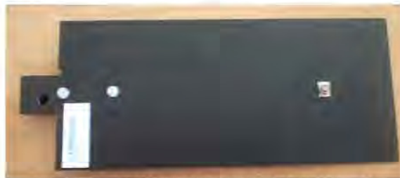
Figure 1 – MVG COMOHAC Validation Dipole
