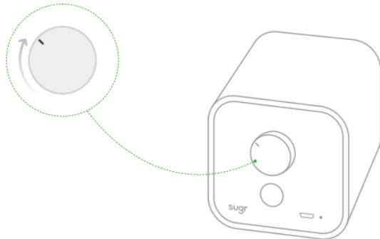
Turn the knob to power on Cube, blue blinking indicates the Discoverable state and the speaker voices "Sugr Cube is now in pairing mode, waiting to pair with your device".
