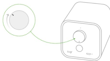
1: Turn the knob of Cube, so the indicator points to the 10 o'clock position.
