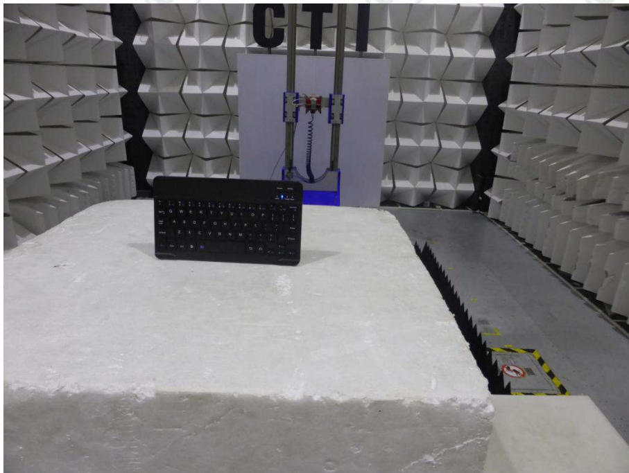
Radiated spurious emission Test Setup-2(Above 1GHz)
