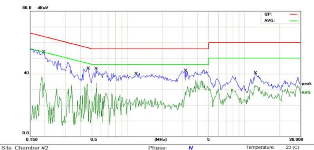
Limit: FCC Part 15B Class B Conduction(QP) Power: AC 230V
