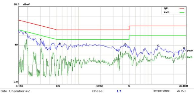
Limit: FCC Part 15B Class B Conduction(QP)
