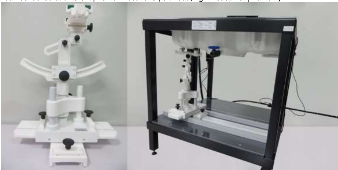
Device holder supplied by SATIMO
