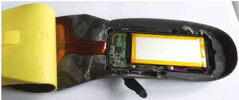
Location of heating pad and electronic box (for small and large sizes)
