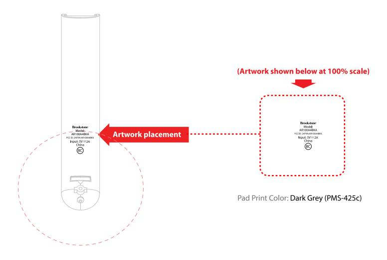
NOTE: The pad print should be placed on the left ear cup and the print should be partially hidden behind the earcup (Indicated by dashed red line) after assembly.
