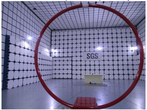
1.3 Radiated Emissions(30MHz-1GHz) Test Setup
