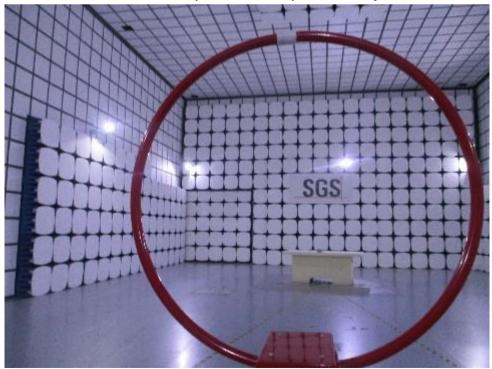
8.2 Radiated Emissions(9kHz-30MHz) Test Setup
