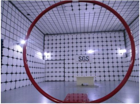
1.3 Radiated Emissions(30MHz-1GHz) Test Setup
