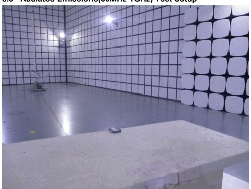
8.3 Radiated Emissions(30MHz-1GHz) Test Setup
