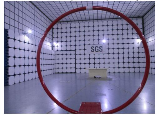
1.3 Radiated Emissions(30MHz-1GHz) Test Setup
