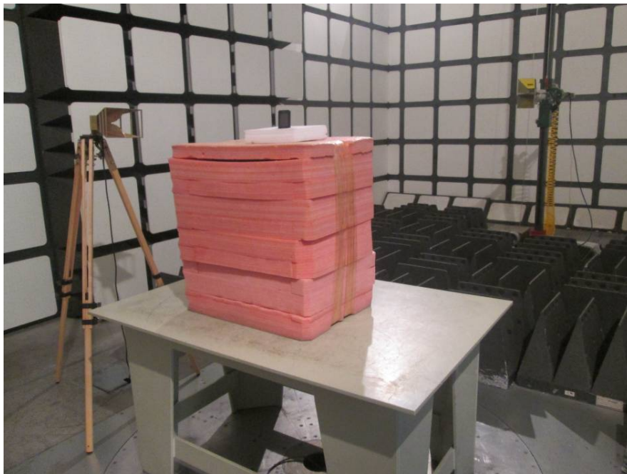
Radiated Emissions Test View (Above 1 GHz)
