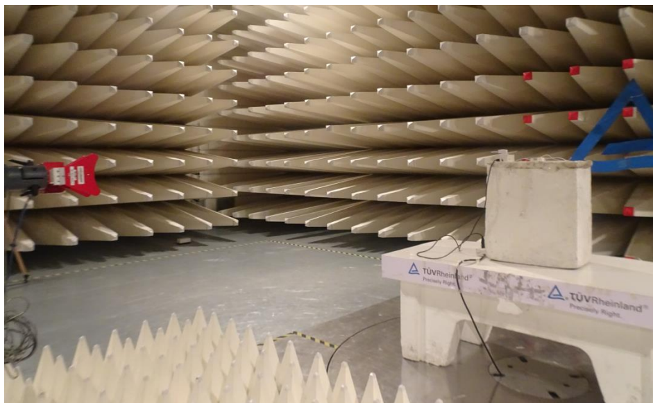
Photo 12: Horn antenna with horizontal polarization
