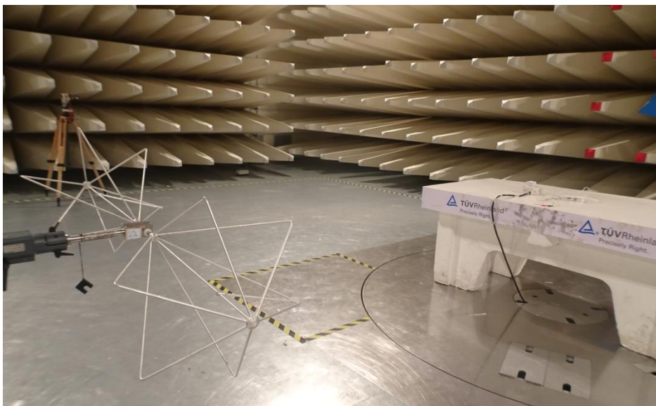
Photo 4: Biconical antenna Horizontal polarization with adapter 2
