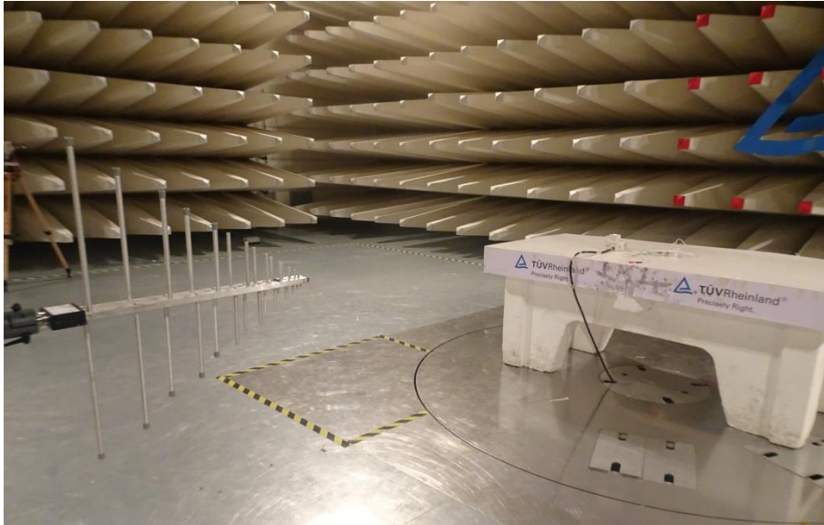
Photo 7: Log periodic antenna Vertical polarization with adapter 2
