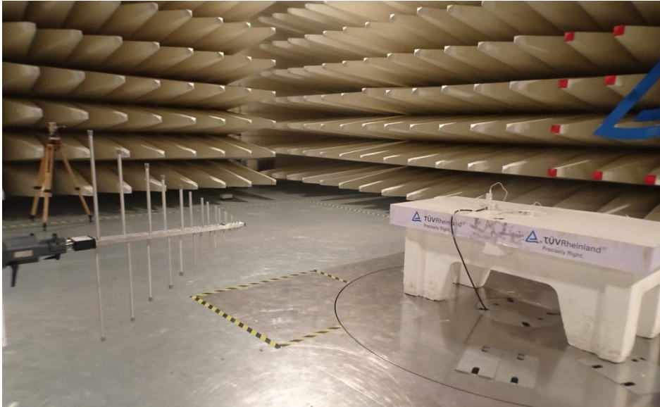
Photo 5: Log periodic antenna Vertical polarization with adapter 1
