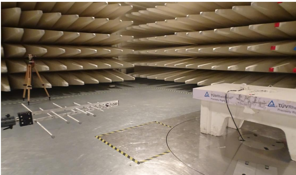
Photo 8: Log Periodic antenna Horizontal polarization with adapter 2
