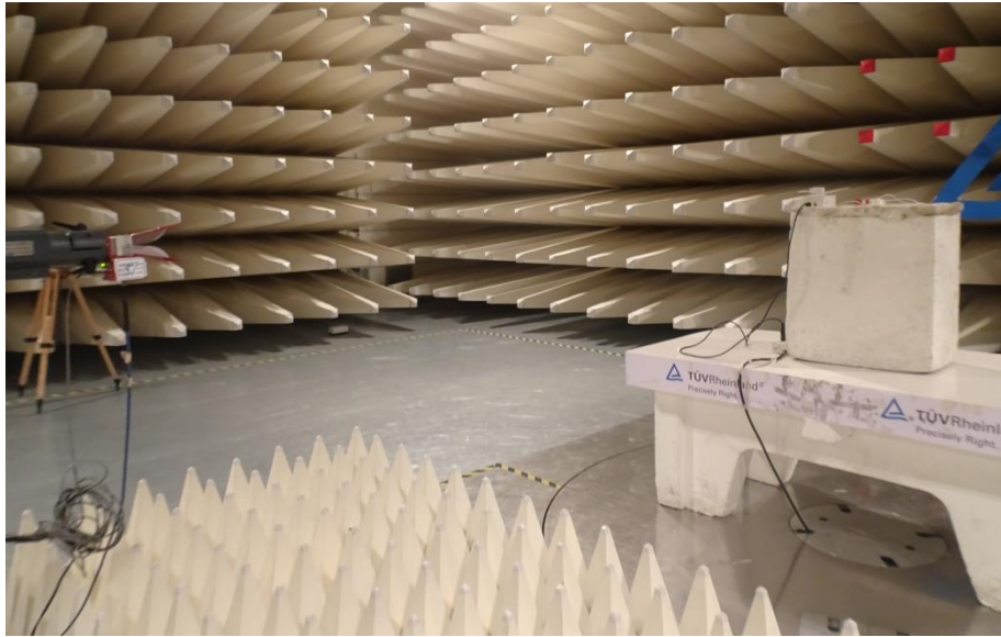
Photo 11: Horn antenna with vertical polarization
