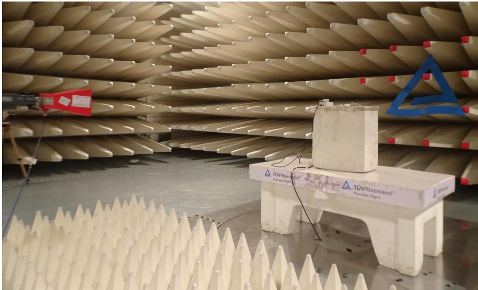
Photo 9: Horn antenna with vertical polarization
