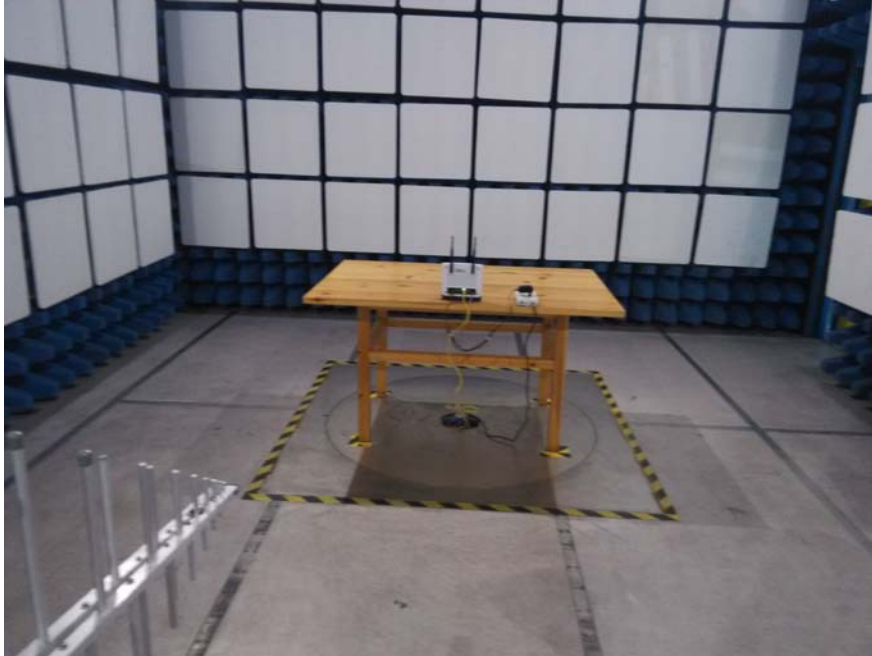
Below 1 GHz, The Normal Working Test Mode
