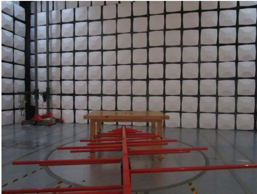
Radiated Emission View (Below 1GHz)
