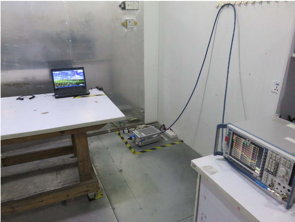
FCC RADIATED EMISSION TEST SETUP
