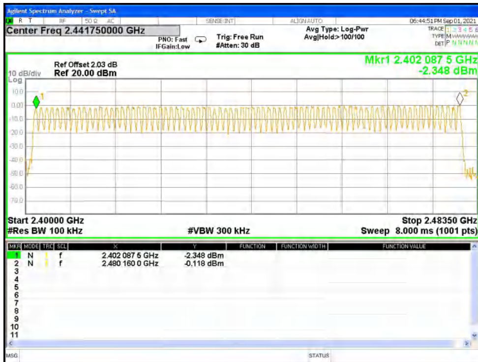
Hopping No. NVNT 1-DH1 2441MHz Ant1
