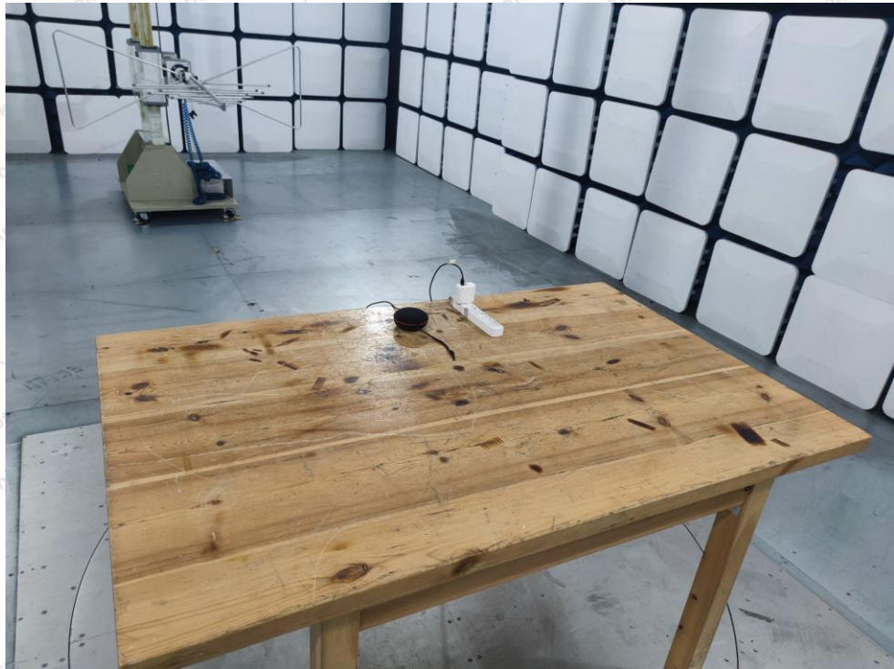
Photo of Radiation Emission Test
