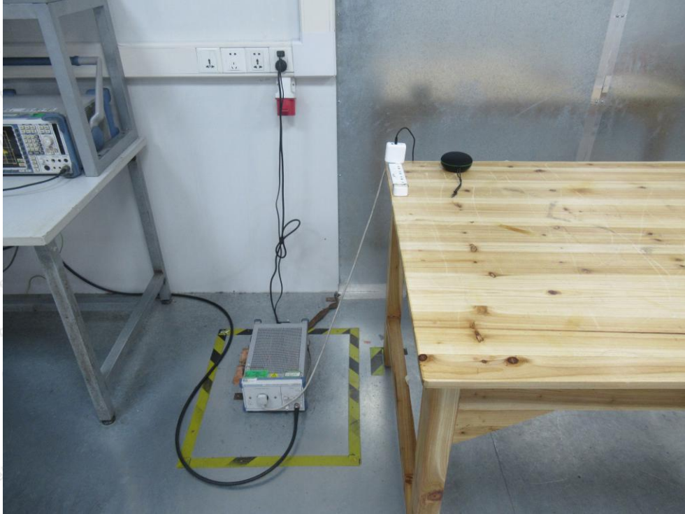
Photo of Conducted Emission Measurement
