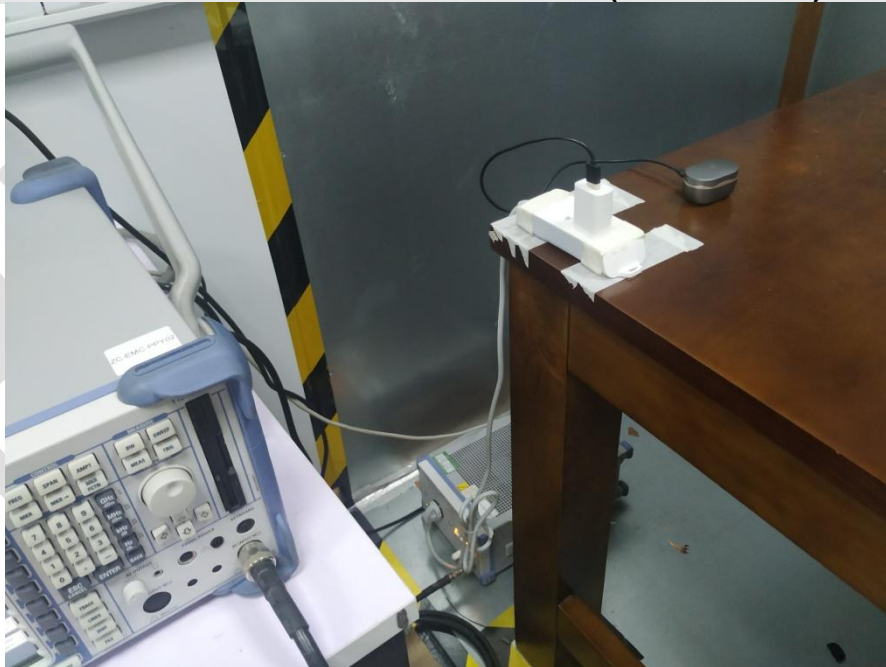
Conducted Emissions at AC Power Line (150kHz-30MHz)
