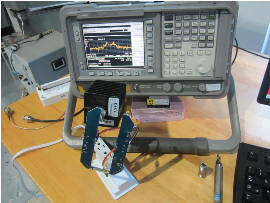
Conducted EMI at the Antenna Port – (915MHz radio)
