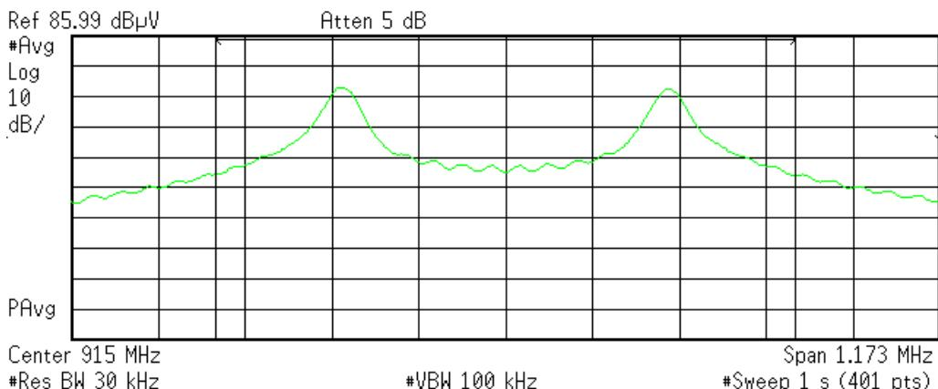
**Channel Power**72.14 dB $\mu$ V/781.9808 kHz**Power Spectral Density**13.20 dB $\mu$ V/Hz**C:\temp.gif file saved**
