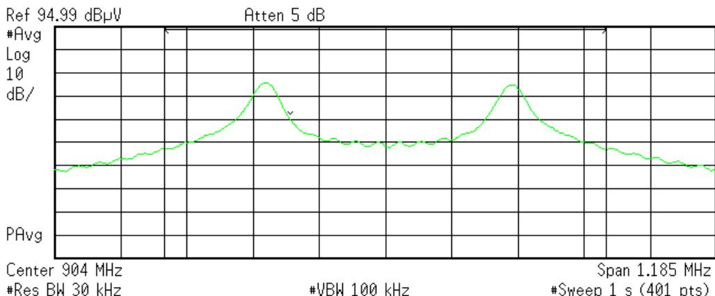
**Channel Power**73.79 dB $\mu$ V/789.4099 kHz**Power Spectral Density**14.82 dB $\mu$ V/Hz**C:\temp.gif file saved**
