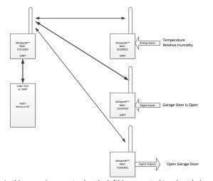
In this example, a master (on the left) is connected to a host (microcontroller or Windows/Linux PC). Three additional modules operate as stand-alone wireless I/O devices. The top right module is connected to analog sensors, the middle right module is using its digital outputs to monitor the state of a garage door, and the lower right module is using its digital output to actually control the garage door.
