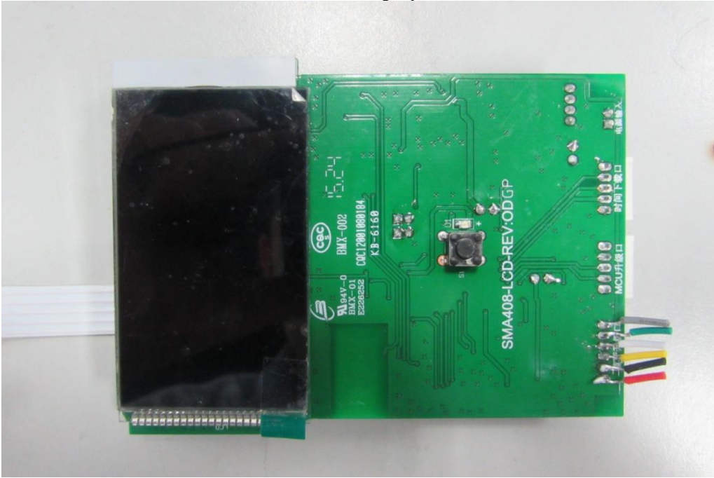
PCB view of display board
