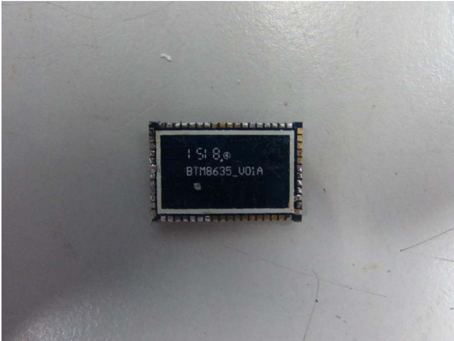
PCB view of Bluetooth module
