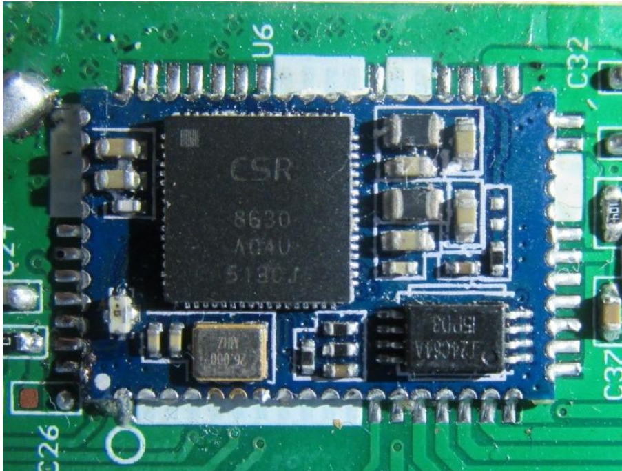
PCB view of Bluetooth module
