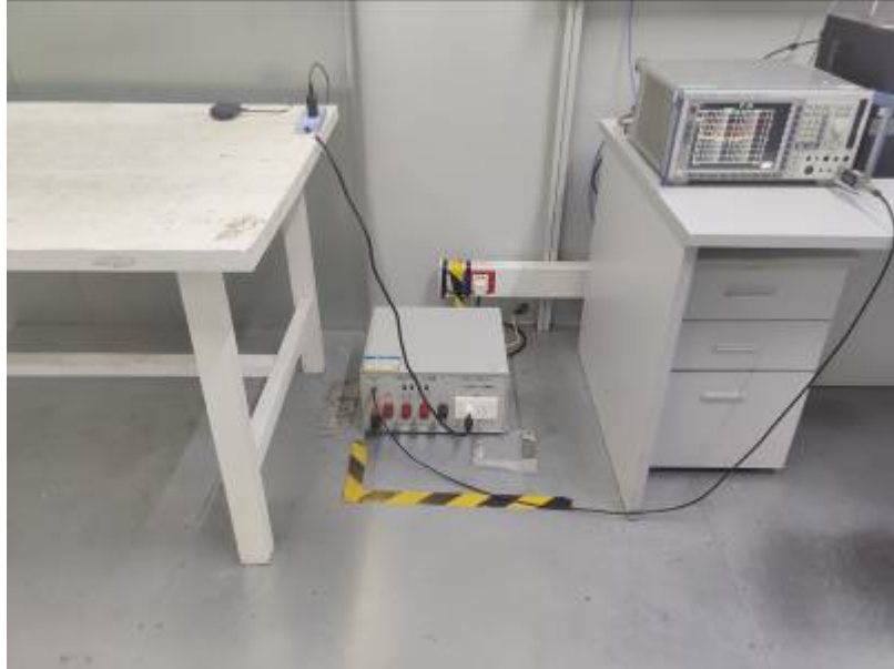
Photos of power line conducted emission test
