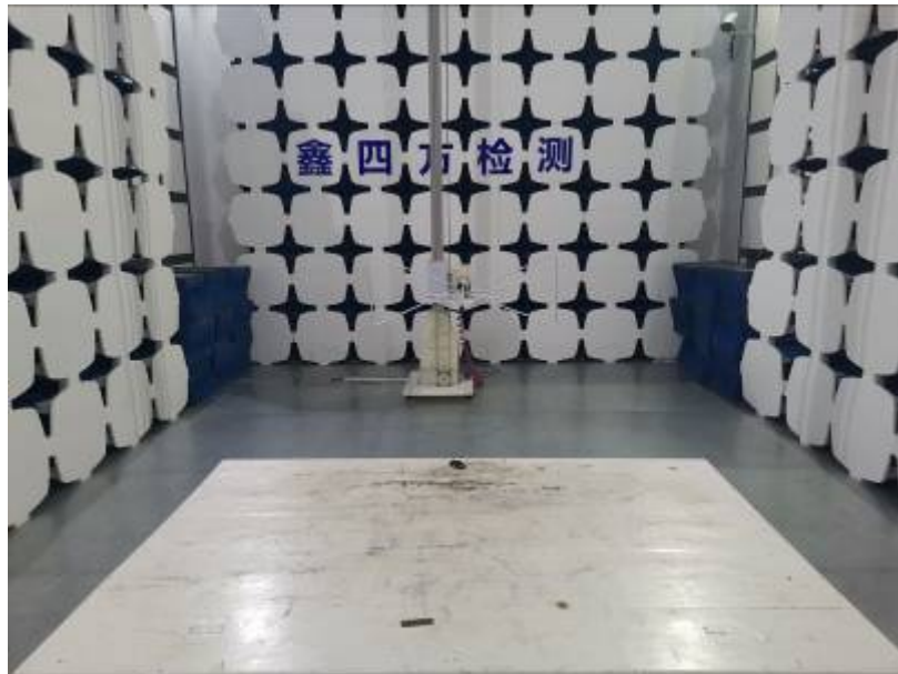
Photos of radiated emission test 30MHz – 1GHz
