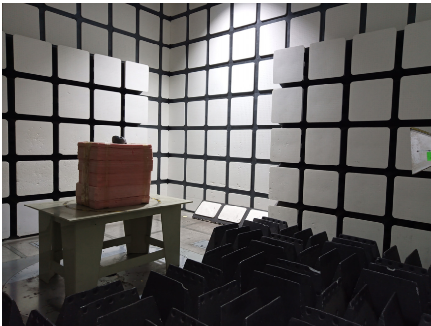
Radiated Emissions View (Above 1 GHz)
