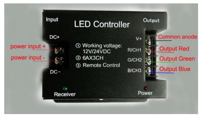
DC+: For power input + (power supply voltage12v-24v)
