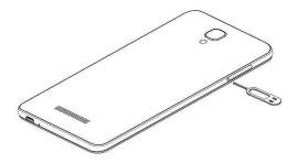
2) Put SIM cards and SD card to card tray correctly.
