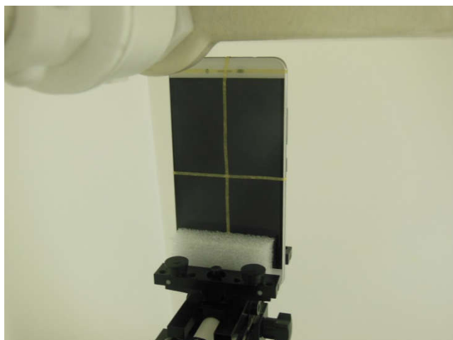
Top Side, Test Separation 10 mm
