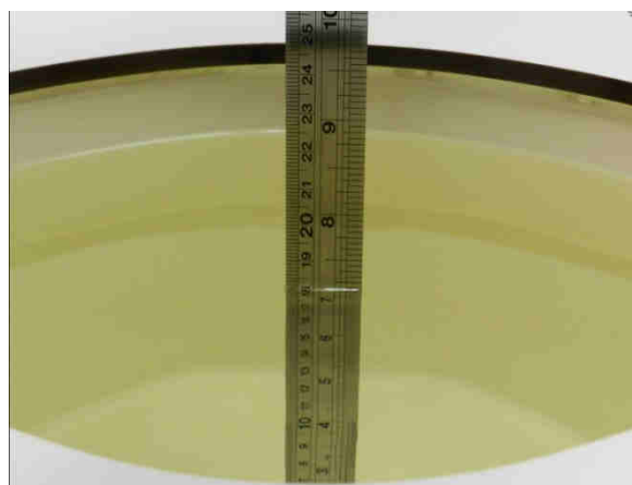
Fig 10.2 Photo of Liquid Height for Body SAR
