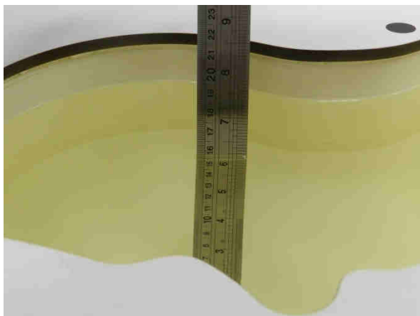
Fig 10.1 Photo of Liquid Height for Head SAR
