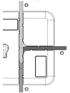
The cable can also descend down through the fixture if a hole or slot is present.
