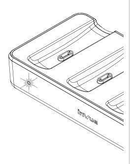
Place a Key onto the contacts in one of the charger slots. Allow the Key to charge for 6 hours before use.
