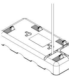
Route the cable as determined in Step 1b, place the charger where desired and apply pressure for at least 10 seconds.
