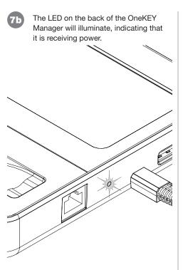
Plug the network cable into the ethernet port on the OneKEY Manager. Follow the screen prompts to set up the OKM
