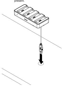
Peel the clear film from the adhesives on the bottom of the charger (4 adhesives on the 4 position charger and 6 on the 8 position charger).
