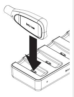
If using the Single Key Charger (OK4101), slide the OneKEY into the charger. Ensure that the charging contacts on the OneKEY align with the charging contacts on the charger.
