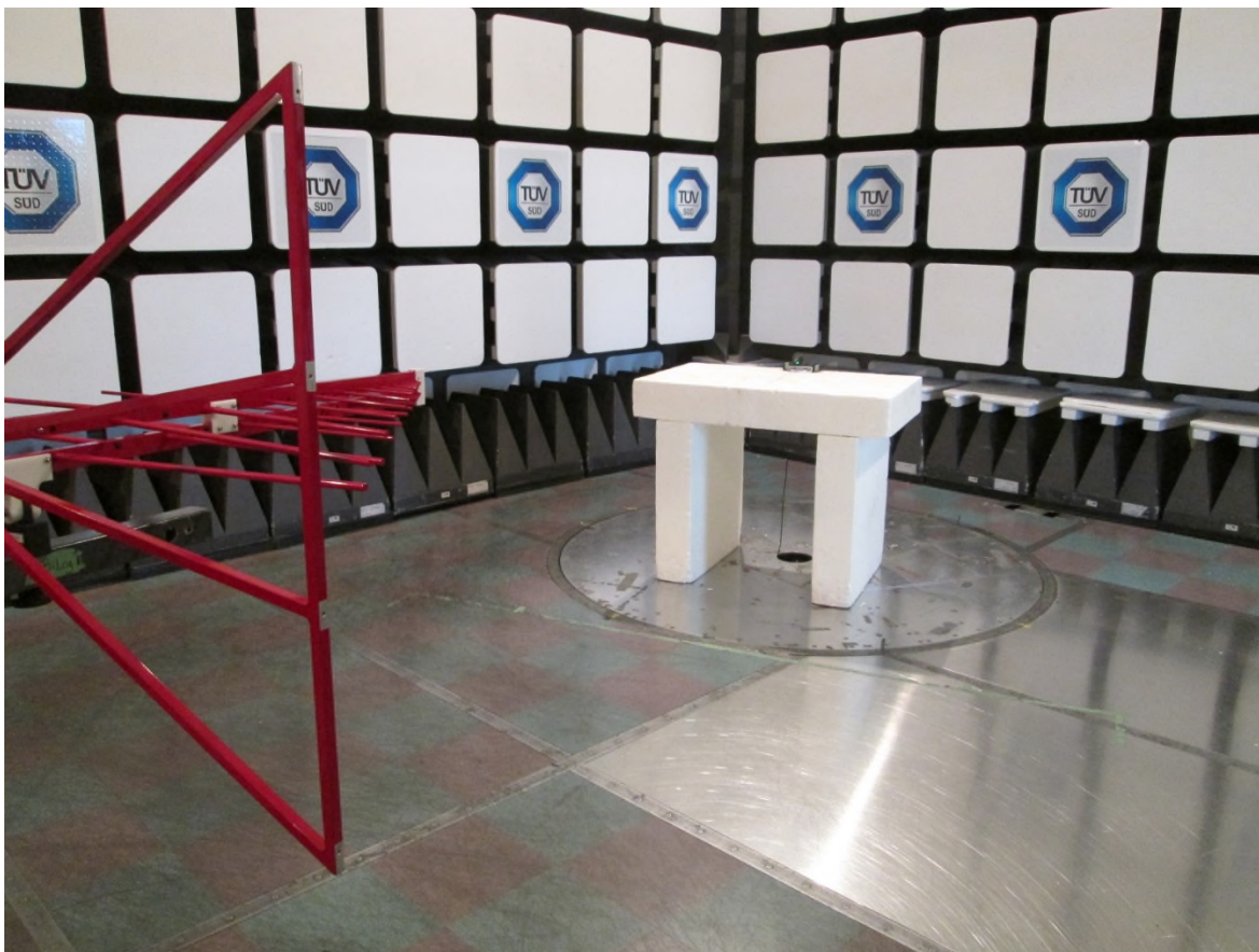
Test setup photo 2 Radiated measurements, 30 MHz – 1 GHz
