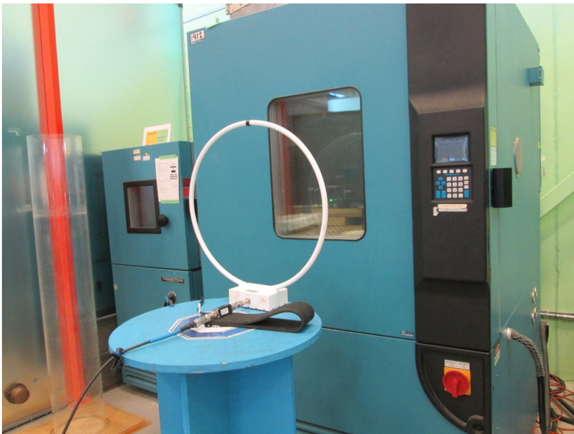
Test setup photo 6 Frequency Stability at Extreme Temperatures, view 1
