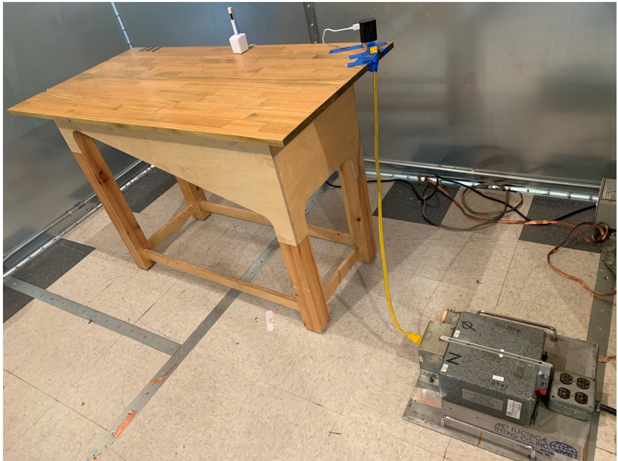
Photograph 1: Conducted Emissions at the Mains Terminal Test Setup
