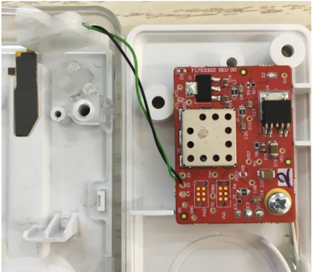
PCBA Top View and Antenna Taken out from Plastic
