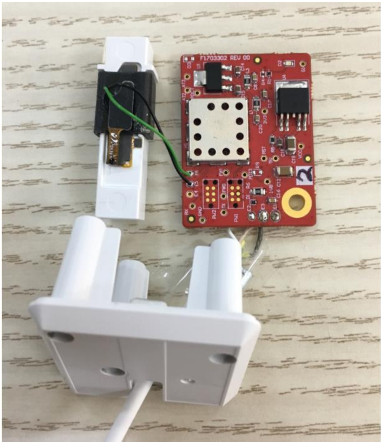
PCBA Top View and Antenna Taken out from Plastic
