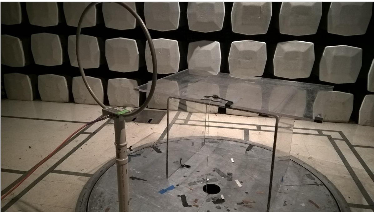
Photograph 2: Radiated Emission, Test Setup, Below 1 GHz
