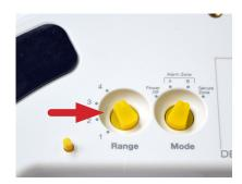
Determine your range settings by consulting the illustration to the right for guidance. Turn the knob to the desired setting by hand or using the key fob tool included with a OneKEY.
