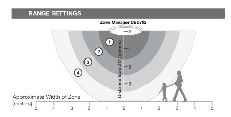
**Note:** All distances are approximate. The shape and distance of the field can be altered by ferrous objects near the Zone Manager (such as structural steel pillars). The field also extends upwards. Keep these factors in mind when installing and setting the range of the field.
