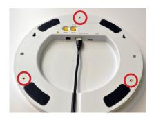
If threading hardware into the M4 x 0.7 threaded inserts on the Zone Manager to install it suspended or against a horizontal surface (ceiling, underside of a table, etc.), ensure that some type of threadlocker (i.e. Loctite Threadlocker Blue) is used. This will prevent loosening through any vibrations.
