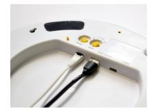
If installing the optional LED Emitter (DBD703), plug that into the 3-pin port in the Zone Manager
