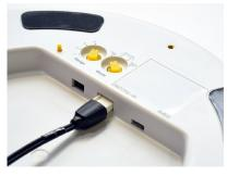
Plug the power supply into the 2-pin port in the Zone Manager.
