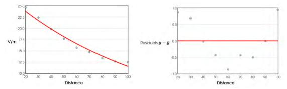
Below is the scatter plot and residual plot for the E-Field measurements.
