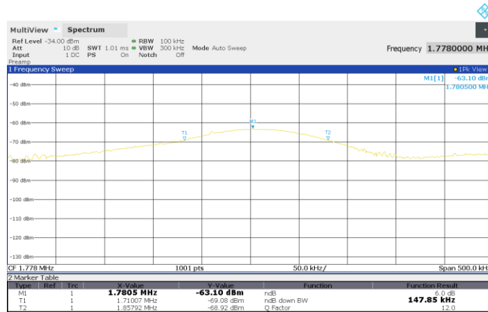
Figure 2.3.6-3: 6 dB Bandwidth – 1.778 MHz
