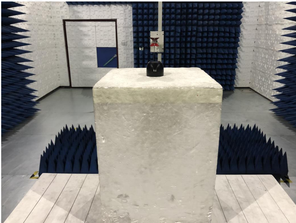
RADIATED EMISSION TEST SETUP ABOVE 1GHZ
