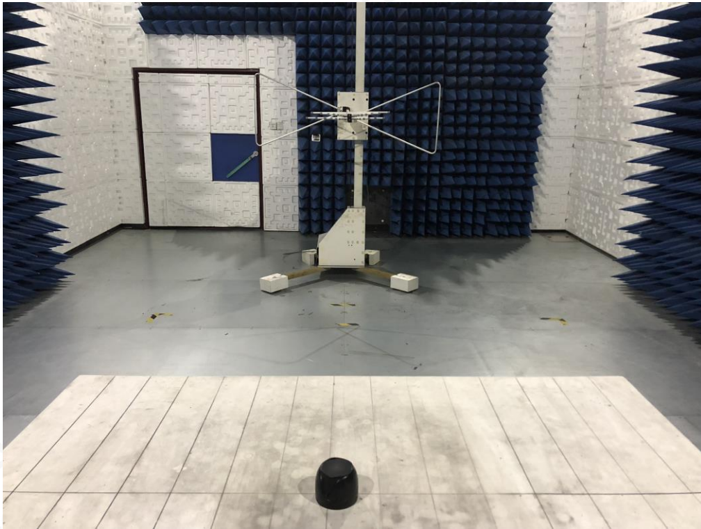
RADIATED EMISSION TEST SETUP ABOVE 1GHZ
