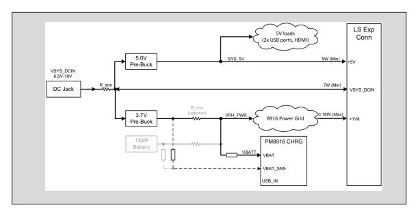
The 96Boards specification defines how power arrives to the board and few supplies that the board needs to provide. The on board power requirement for each 96Boards implementation depends on the SoC and the set of peripherals that are specific to that implementation.
