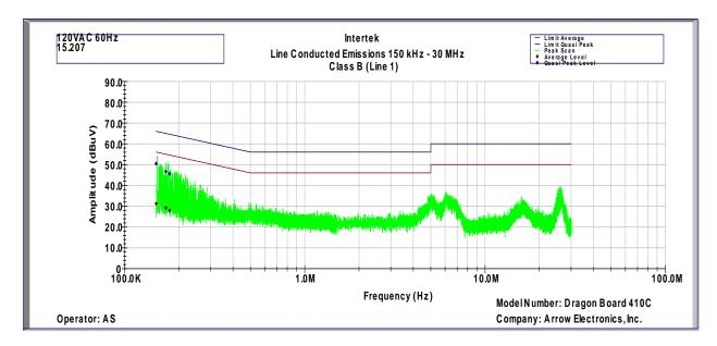
Intertek Testing Services Line Conducted Emissions 150 kHz - 30 MHz
