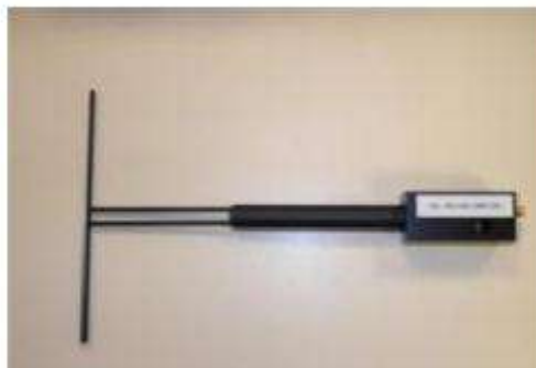
Figure 1 – Satimo COMOSAR Validation Dipole
