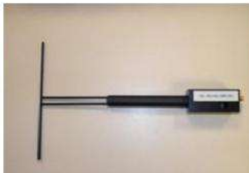
Figure 1 – Satimo COMOSAR Validation Dipole
