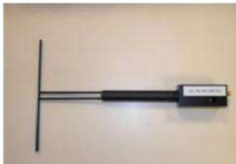
Figure 1 – Satimo COMOSAR Validation Dipole
