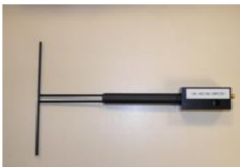
Figure 1 – Satimo COMOSAR Validation Dipole
