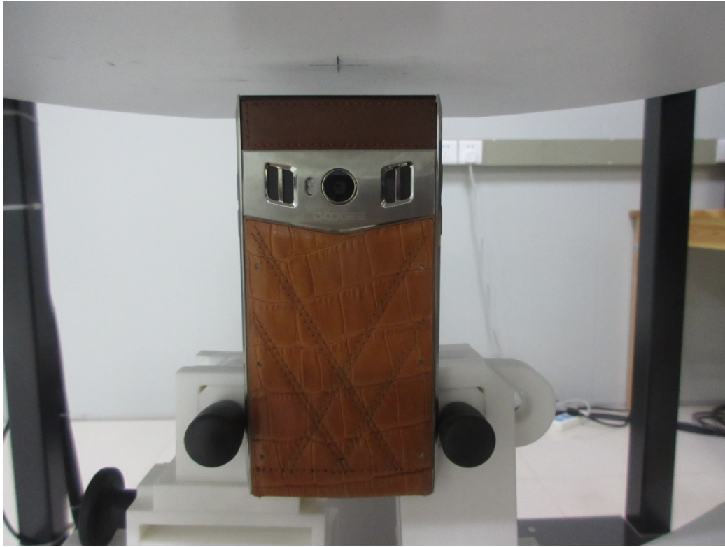
10mm body-worn Top Side Setup Photo(hotspot)
