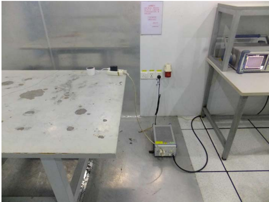
1 Photo of Power Line Conducted Emission Measurement
